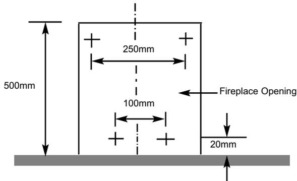
Fit the wallplugs provided and screw the fixing eyes securely into the rear of the fire opening. If the clearance at the rear of the fire is at the minimum specified for a precast flue application, it may be necessary to bend over the lower fixing eyes after screwing them fully in to the rear of a pre-cast starter block.
